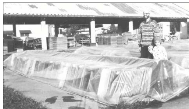
A high-humidity easy-access solar curing chamber
